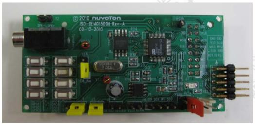
Figure 1 – Top view of ISD-DEMO15D00 Rev-A board
