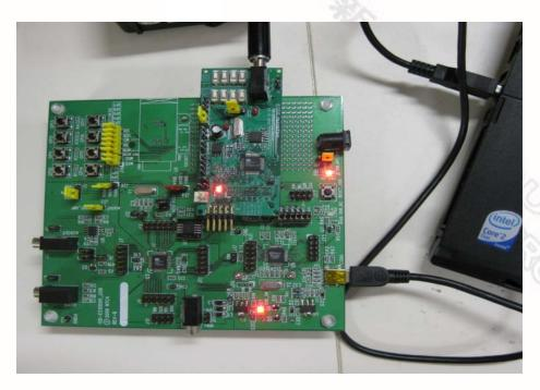
Figure 6 - ISD15D00 is connected onto ISD-ES15D00\_USB mother board
