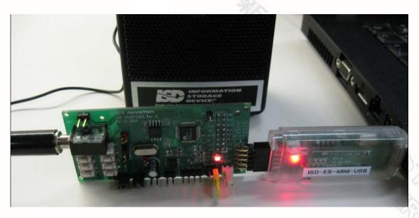
Figure 4 – A complete evaluation environment for ISD15D00 device
