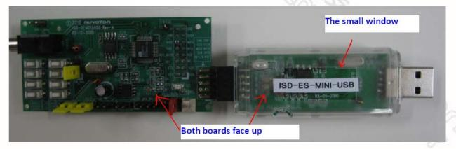
Figure 5 – connect ISD15D00 demo board with the USB dongle.
