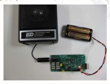
Figure 8 – ISD15D00 demo board standalone evaluation.
