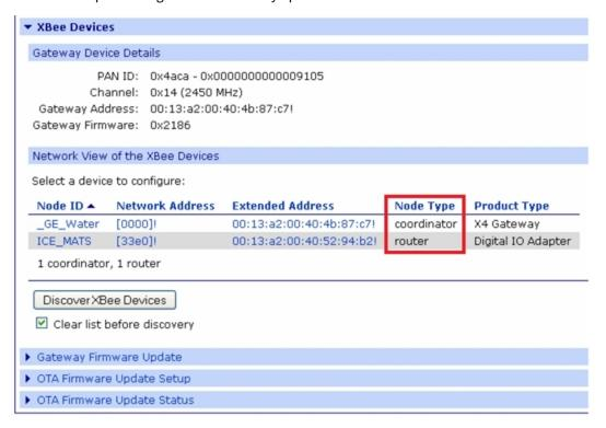
XBee 802.15.4 series products show all nodes as **end nodes** by default. You can set one node in the network as **coordinator**, as in the following example:
