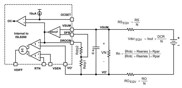
FIGURE 47. EQUIVALENT MODEL FOR DROOP AND DIE SENSING USING DCR SENSING
