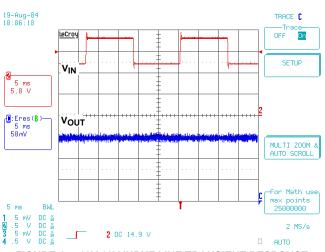
FIGURE 15. 12V-18V INPUT LINE TRANSIENT RESPONSE
