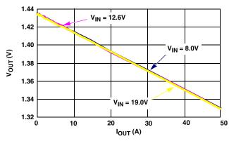
FIGURE 10. ACTIVE MODE LOAD LINE, 2 PHASE, CCM, PSI# = HIGH, VID = 1.435V
