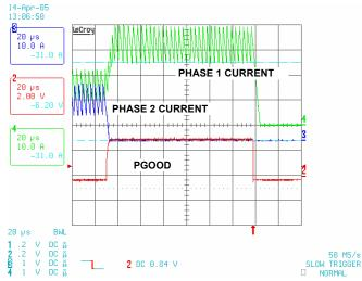
FIGURE 34. ISL6260C, OVERCURRENT DUE TO PHASE DROPPING
