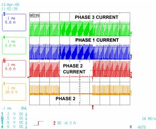
FIGURE 32. ISL6260C, INDUCTOR CURRENT WAVEFORM
