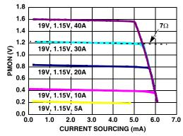
FIGURE 35. POWER MONITOR CURRENT SOURCING CAPABILITY
