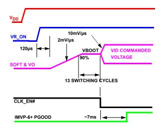
FIGURE 42. SOFT-START WAVEFORMS USING A 20nF SOFT CAPACITOR
