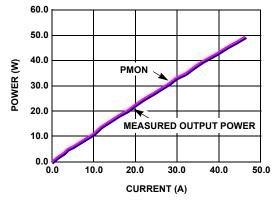
FIGURE 38. POWER MONITOR vs OUTPUT CURRENT
