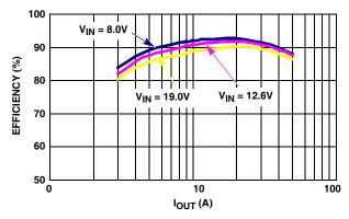
FIGURE 7. ACTIVE MODE EFFICIENCY, 2 PHASE, CCM, PSI# = HIGH, VID = 1.4375V
