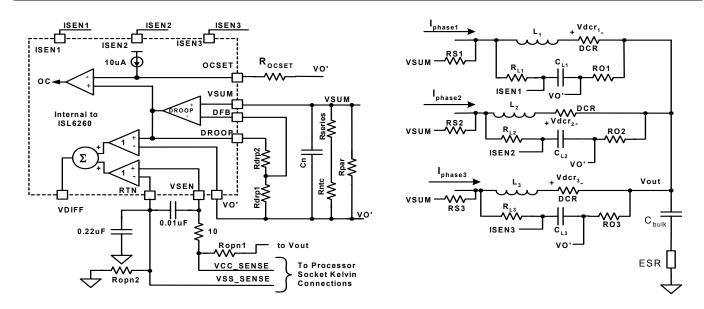
FIGURE 46. EQUIVALENT MODEL FOR DROOP AND DIE SENSING USING DCR SENSING
