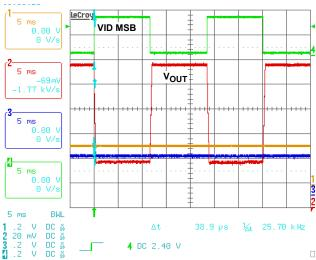
FIGURE 24. SLEW RATE ENTERING C4, VID MSB BIT CHANGE FROM 1.4375V TO 0.65V SHOWING 2mV/µs SLEW RATE, DPRSLPVR = 1, DPRSTP# = 0
