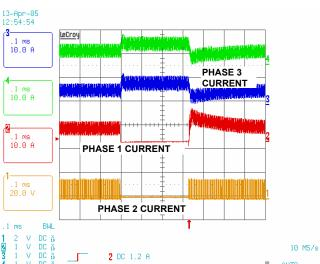
FIGURE 33. ISL6260C, INDUCTOR CURRENT WAVEFORM
