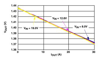
FIGURE 4. DEEPER SLEEP MODE LOAD LINE, 3 PHASE, CCM, PSI# = LOW VID = 1.435V
