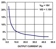
FIGURE 37. POWER MONITOR ACCURACY
