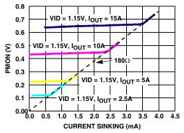
FIGURE 36. POWER MONITOR CURRENT SINKING CAPABILITY
