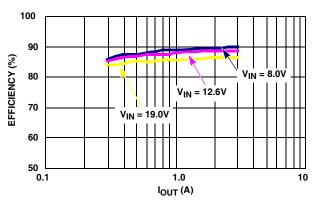
FIGURE 8. DEEPER SLEEP MODE EFFICIENCY, 2 PHASE, DCM OPERATION, PSI# = LOW, VID = 1.4375V
