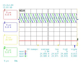
FIGURE 18. 2 PHASE CURRENT BALANCE, FULL LOAD = 50A
