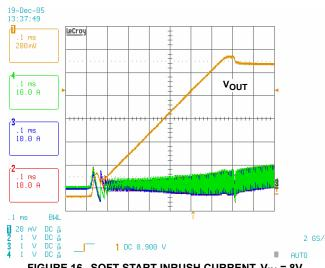
FIGURE 16. SOFT-START INRUSH CURRENT,  $V_{IN} = 8V$
