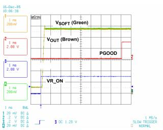
FIGURE 14. SOFT-START WAVEFORM SHOWING PGOOD
