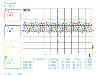
FIGURE 17. 3 PHASE CURRENT BALANCE, FULL LOAD = 50A
