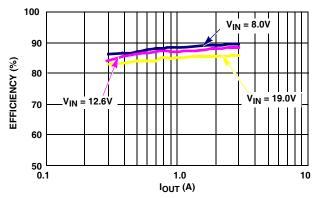
FIGURE 3. DEEPER SLEEP MODE EFFICIENCY, 3 PHASE, DCM OPERATION, PSI# = LOW, VID = 1.4375V
