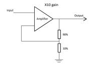
With an infinite gain the amplifier is no good to amplify audio, which is where the feedback comes in. By making one of the inputs a percentage of the output the gain can be fixed, which allows the output to be a copy of the input but bigger. Now when the two inputs are compared and the output is adjusted, instead of it going up or down until it reaches 0 volts or V+, it stops at the point when the two inputs match and the output is at the required voltage.
