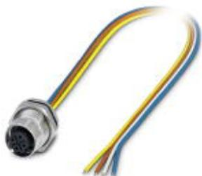
Bus system flush-type socket, PROFINET, 4-pos., M12 SPEEDCON, D-coded, front/screw mounting with Pg9 thread, with 0.5 m TPE litz wire, 4 x 0.34 mm<sup>2</sup>
