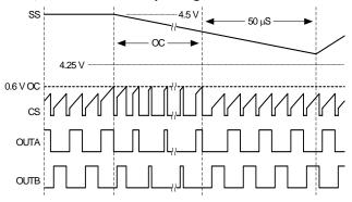
FIGURE 9. OC RECOVERY PRIOR TO SHUTDOWN
