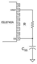
FIGURE 10. MODIFYING OC SHUTDOWN TIMING
