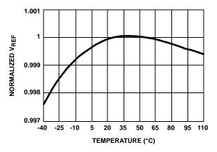
FIGURE 1. REFERENCE VOLTAGE vs TEMPERATURE
