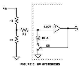
As  $V_{IN}$  decreases to a UV condition, the threshold level is:  $V_{IN(DOWN)} = \frac{R1+R2}{R2} \qquad V \tag{EQ. 7}$
