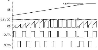
FIGURE 7. PULSE-BY-PULSE OC BEHAVIOR DURING SS
