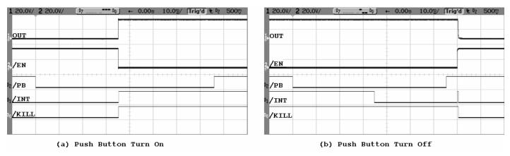
Figure 2. Push Button Turn On/Off with ONT and PDT Open (time scale at 10ms/div)
