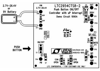
Figure 1. DC1090A Example Setup
