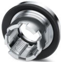
M12 threaded sleeve with tolerance-compensating function, for straight, SMD-solderable M12 socket contact inserts. Suitable for 1.6 mm ... 2.3 mm thick front plates.
