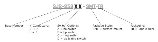
Note: 1. 2 conductor option only available with tip switch
