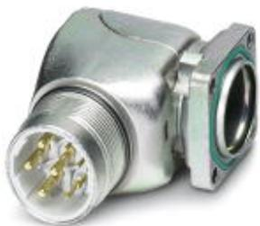
Device connector, front mounting, angled rotatable, Screw locking, M23, Number of positions: 4+3+PE, Type of contact: Pin, Crimp connection, Axial O-ring, 4x Ø 3.2, shielded: yes, Flange dimensions: 28 mm x 28 mm, Compatible with mating connectors with SPEEDCON or M23 standard knurled nuts
