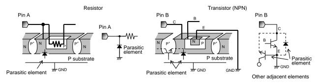
Fig.3 Pattern Diagram of Parasitic Element
