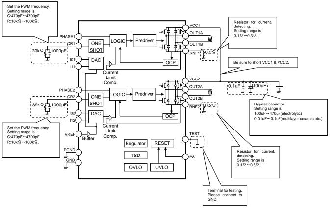
Fig.1 Block diagram & Application circuit diagram
