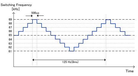
Figure 10. Frequency hopping function
