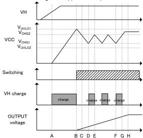
Figure 9. Charge operation VCC pin charge operation
