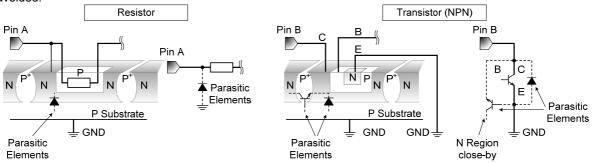
Figure 18. Example of monolithic IC structure
