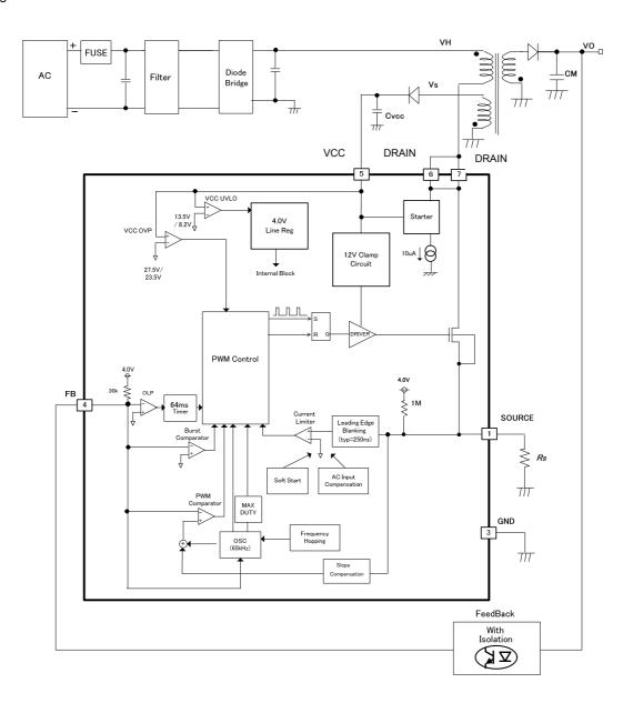
Figure 3. Block Diagram
