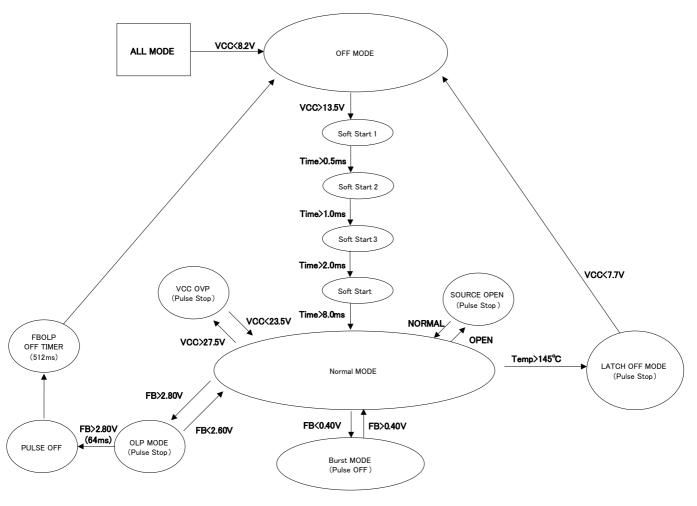
Figure 16. The sequence diagram
