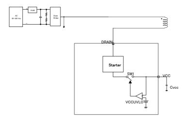
Figure 4. Block diagram of start circuit
