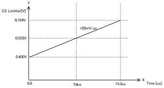
Figure 14. Over current limiter voltage
