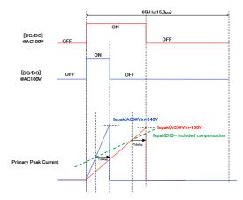
Figure 12. No AC voltage compensation function
