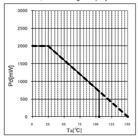
Figure 17. DIP7 Thermal Abatement Characteristics
