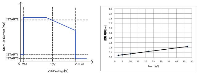
Figure 5. Start current vs VCC voltage
