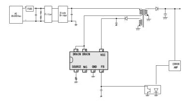
Figure 1. Application circuit
