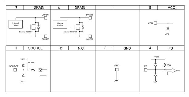
Figure 2 I/O Equivalent Circuit Diagram
