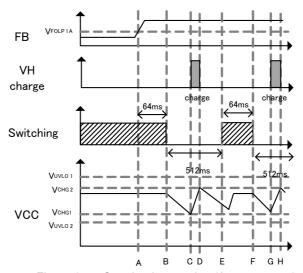
Figure 15. Over load protection (Auto recovery)
