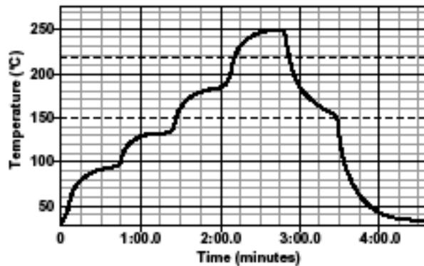
**Figure 3. Lead-free (SnAgCu) Solder Ball Reflow Profile**
