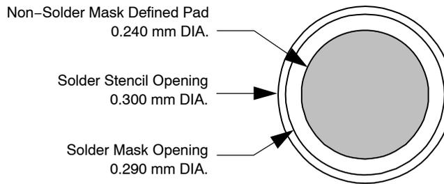
**Figure 2. Recommended Non-Solder Mask Defined Pad Illustration**
