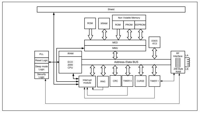
Figure 2: Block Diagram of SLE 66CL81P
