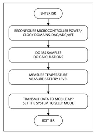
Figure 5. MAXREFDES73# firmware interrupt service routine flowchart.
