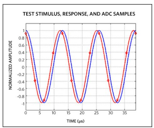
Figure 3. MAXREFDES73# ADC quadrature sampling.
