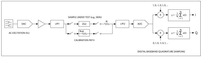
Figure 2. MAXREFDES73# AC impedance measurement block diagram.
