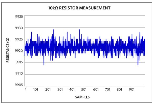
Figure 7. MAXREFDES73# 10kΩ resistor measurement.
