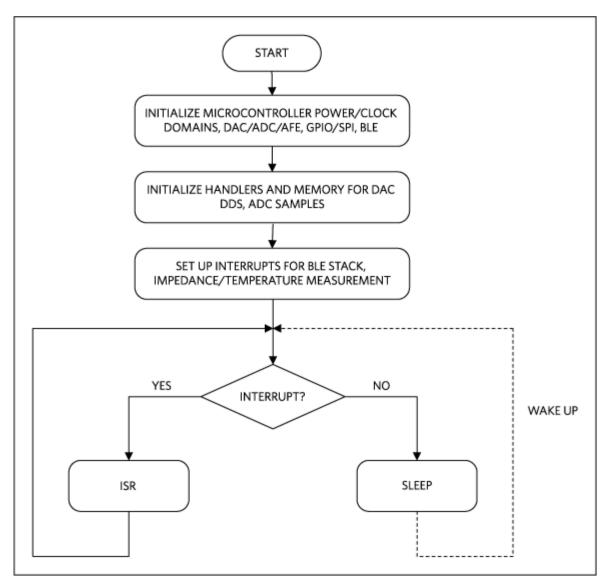
Figure 4. MAXREFDES73# firmware main function flowchart.
