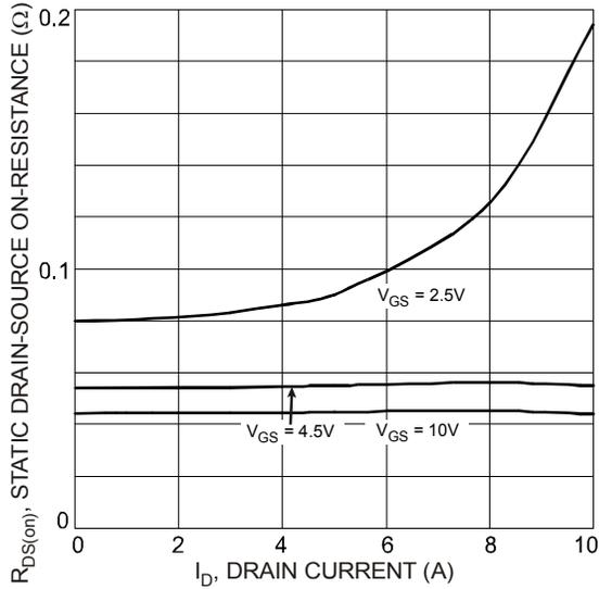
Fig. 3 On-Resistance vs. Drain Current and Gate Voltage
