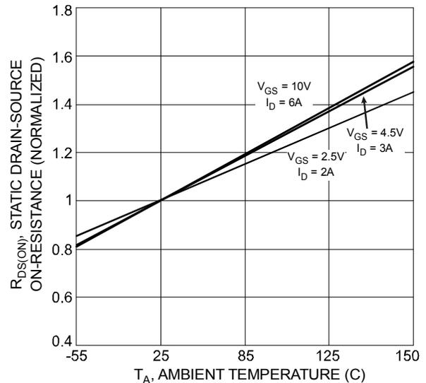
Fig. 6 Normalized Static Drain-Source On-Resistance vs. Ambient Temperature
