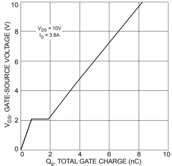
Fig. 8 Gate-Source Voltage vs. Total Gate Charge
