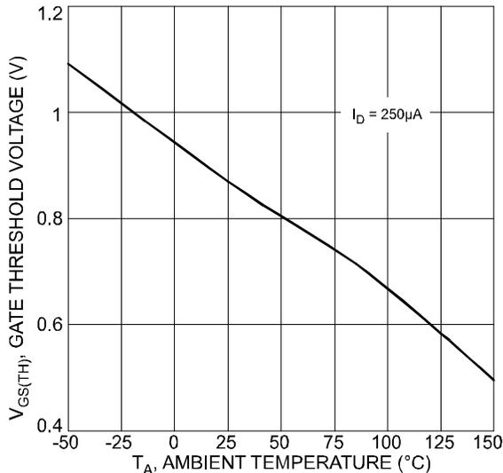
Fig. 5 Gate Threshold Voltage vs. Ambient Temperature
