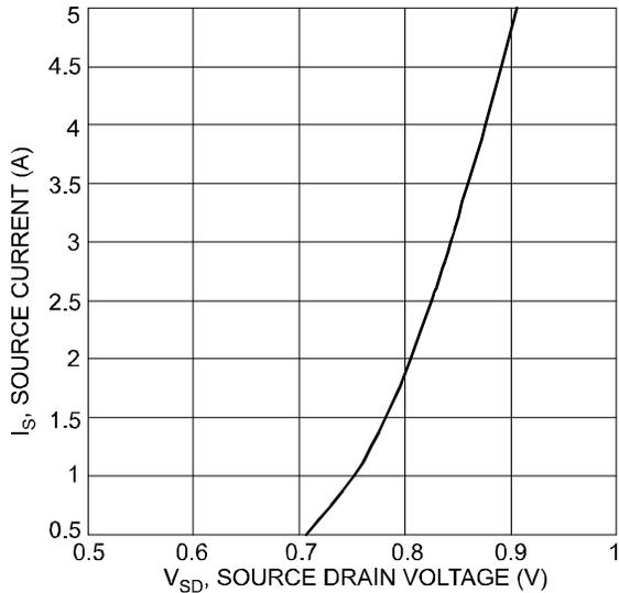
Fig. 7 Reverse Drain Current vs. Source-Drain Voltage
