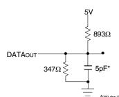
Figure 1. AC Output Test Load
