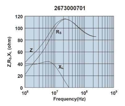
Impedance, reactance, and resistance vs. frequency.
