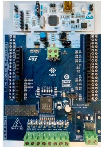
X-NUCLEO-OUT01A1 plugged on to a compatible STM32Nucleo board
