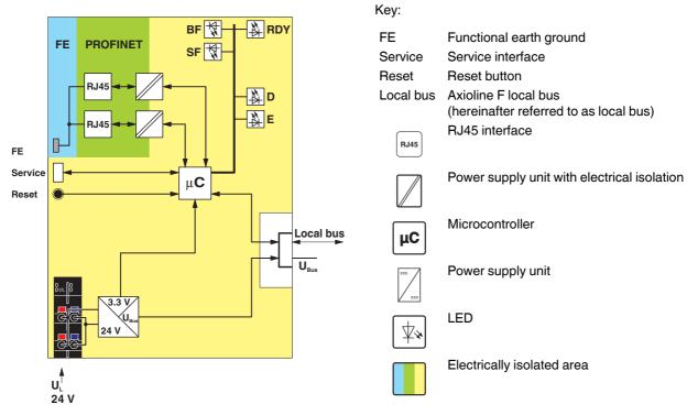
Figure 1 Internal wiring of the terminal points
