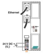
Figure 4 Connection of the cables
