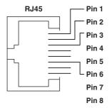
Figure 2 Pin assignment of the Ethernet socket (RJ45)
