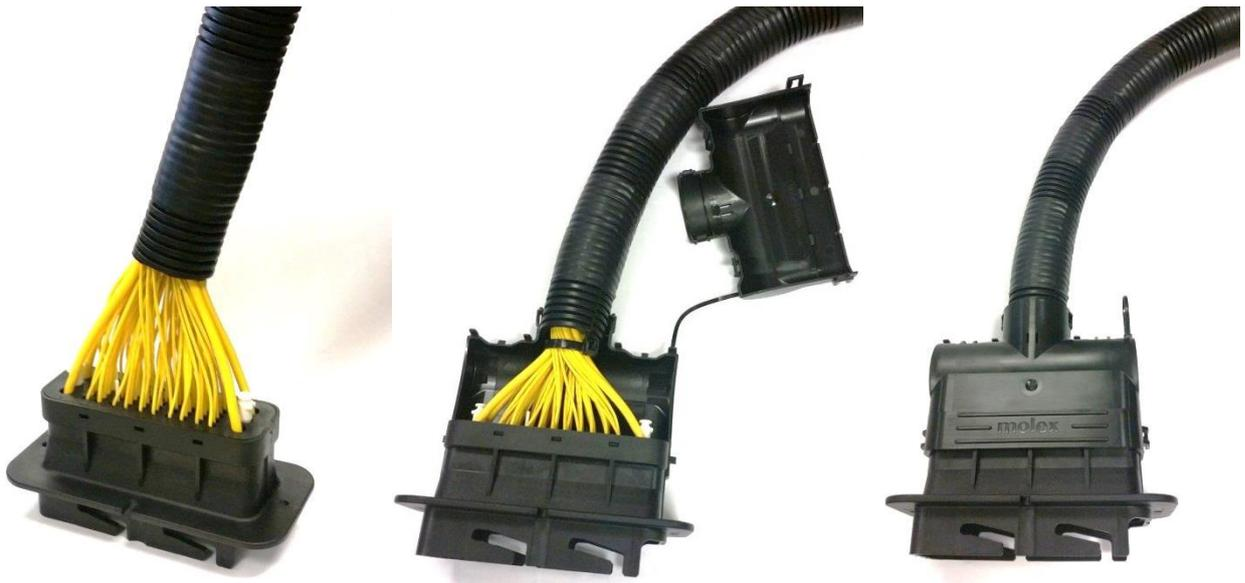
Figure 4.34: (Left) A fully-assembled SRC Male Connector Assembly with conduit around the wires, (Middle) one half of the Conduit Interface assembled with a tie wrap used as strain relief on the cables and (Right) a correctly assembled conduit to a SRC Male Connector using the appropriate Conduit Interface
