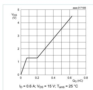
Fig. 16. TR1: Gate-source voltage as a function of gate charge; typical values
