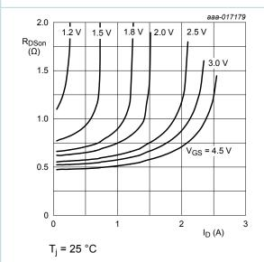
Fig. 10. TR1: Drain-source on-state resistance as a function of drain current; typical values
