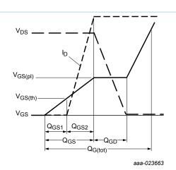
Fig. 17. TR1: Gate charge waveform definitions
