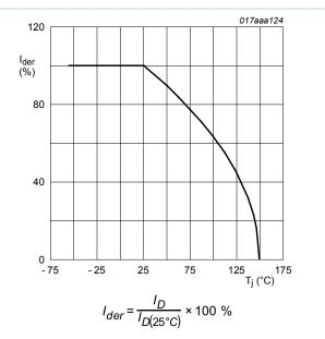
Fig. 3. MOSFET transistor: Normalized continuous drain current as a function of junction temperature
