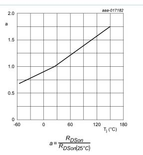
Fig. 13. TR1: Normalized drain-source on-state resistance as a function of junction temperature; typical values
