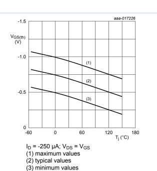
Fig. 25. TR2: Gate-source threshold voltage as a function of junction temperature
