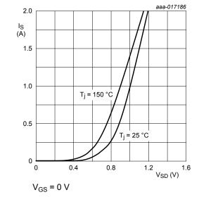
Fig. 18. TR1: Source current as a function of sourcedrain voltage; typical values
