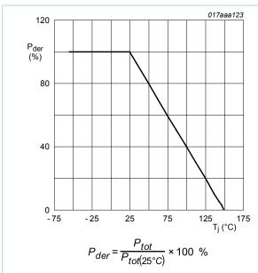
Fig. 2. MOSFET transistor: Normalized total power dissipation as a function of junction temperature
