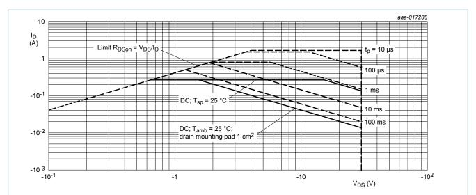
Fig. 5. TR2: Safe operating area; junction to ambient; continuous and peak drain currents as a function of drain-source voltage
