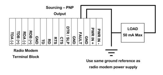
Figure 4-9 Fault Output Wiring
