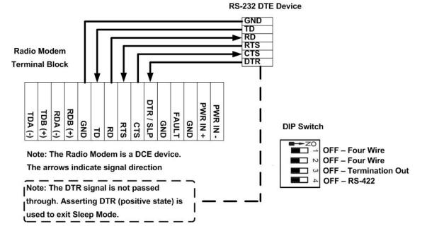
Figure 4-3 RS-232 Wiring
