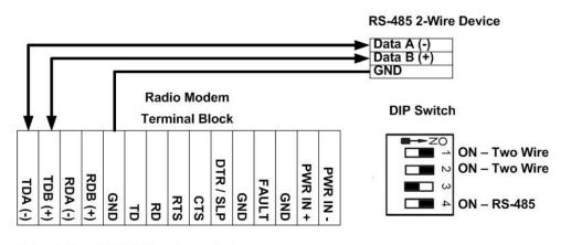
Note: A (-) and B (+) Signals are tied together when the DIP Switch is configured to 2-Wire Mode.
