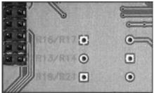
Figure 4-6 Through-hole Resistor Pads
