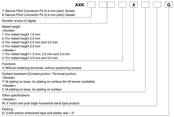
Notes: 1. Only a socket of mated height 3.5 mm: 2,000 pieces embossed tape and plastic reel  $\times$  2.
