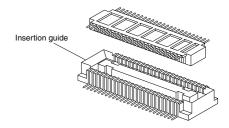
3) Simple lock structure provides tactile feedback to ensure excellent mating/ unmating operation feel.
