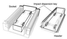
A high level of shock resistance is ensured by dispersing impact over the four locations where the socket indentations and header protrusions are mated together.
