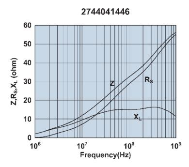
Impedance, reactance, and resistance vs. frequency.
