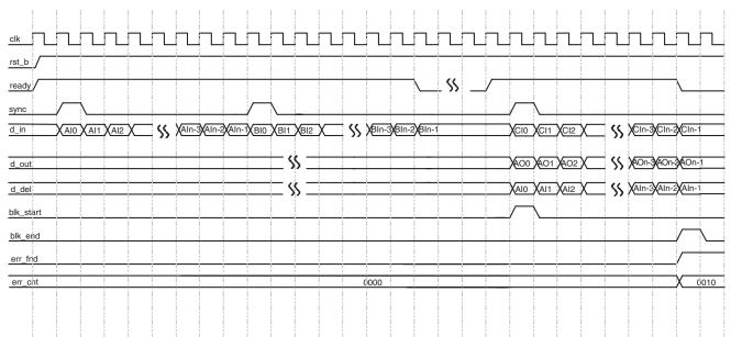
Figure 4 illustrates the output status when sr is asserted. When sr is asserted during the decoding process, it reinitializes the decoder state. It forces the data at d\_in to be output to d\_out without correction.
