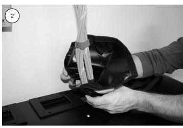
Step 2: Place the fitting around the cable bundle.
