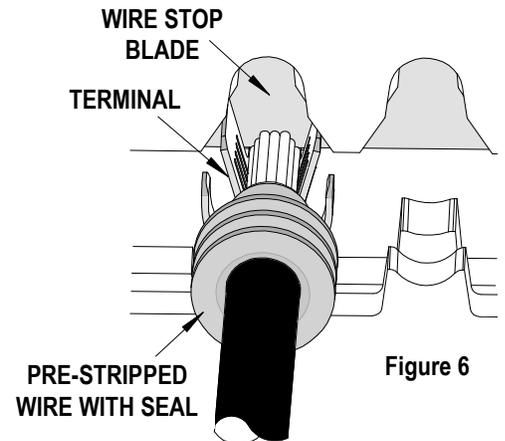
10. Compress the terminal by squeezing the tool handles until the ratchet mechanism cycle has been completed. Release handles to open the jaws.
