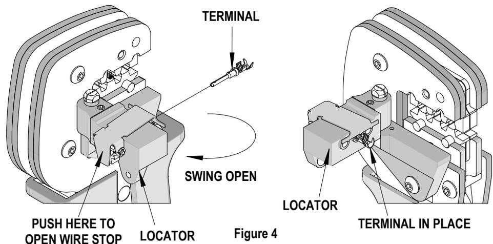
7. Turn the Locator Lock Latch up to lock. Make sure that the terminal is visually centered over the punch.
