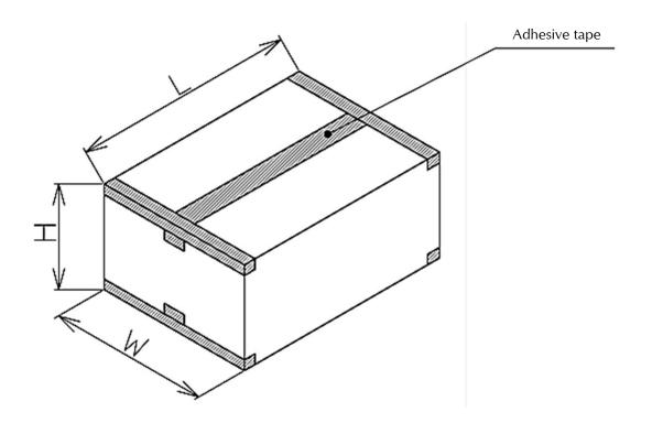
Note a. The above figure is a representative example. The way that how adhesive tape is applied on the box differs by the box type.
