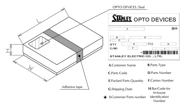
Notes a. The above figure is a representative example. The way that how adhesive tape is applied differs by the box type.
