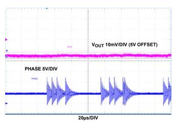
FIGURE 14. NON-SYNCHRONOUS BUCK, FORCE PWM MODE,  $V_{\mbox{\scriptsize IN}}$  12V, NO LOAD
