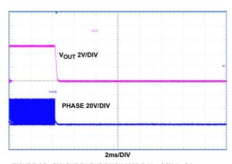
FIGURE 12. SYNCHRONOUS BUCK MODE,  $V_{\mbox{\scriptsize IN}}$  36V,  $I_{\mbox{\scriptsize O}}$  2A, ENABLE OFF
