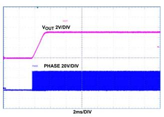
FIGURE 10. SYNCHRONOUS BUCK MODE,  $V_{\mbox{\footnotesize IN}}$  36V,  $I_{\mbox{\footnotesize O}}$  2A, ENABLE ON
