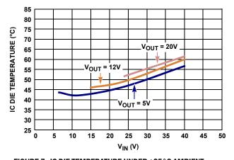
FIGURE 7. IC DIE TEMPERATURE UNDER +25 °C AMBIENT TEMPERATURE, STILL AIR, 500kHz,  $I_0$  = 2A
