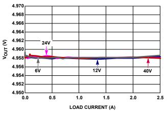
FIGURE 5. LOAD REGULATION,  $V_{OUT}$  5V,  $T_A = +25 \,^{\circ}$  C
