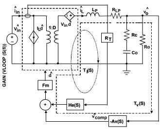
FIGURE 18. SMALL SIGNAL MODEL OF BUCK REGULATOR
