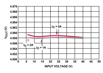
FIGURE 6. LINE REGULATION,  $V_{OUT}$  5V,  $T_A$  = +25°C
