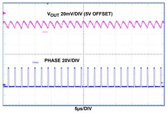
FIGURE 11. SYNCHRONOUS BUCK,  $V_{\mbox{\scriptsize IN}}$  36V,  $I_{\mbox{\scriptsize O}}$  2A
