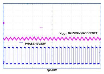
FIGURE 15. NON-SYNCHRONOUS BUCK, FORCE PWM MODE,  $V_{\mbox{\scriptsize IN}}$  12V, 2A
