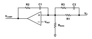
FIGURE 19. TYPE III COMPENSATOR
