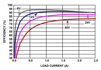
FIGURE 4. EFFICIENCY, SYNCHRONOUS BUCK, 500kHz, V<sub>OUT</sub> 3.3V, T<sub>A</sub> = +25°C
