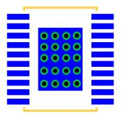
FIGURE 21. PCB VIA PATTERN
