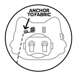
Go through the same steps that you did for the first badge hook with the first of the sensor's hooks: anchor the thread, wrap it four or five times around the hook, then anchor again.
