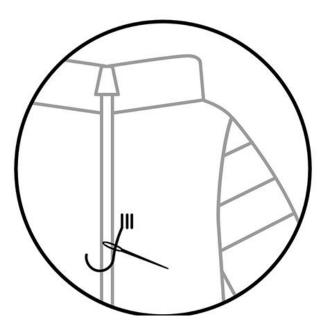
Using your needle, loop the thread around the first hook four or 5 times, pulling it tight against the fabric and making sure that it's tightly wound round the hook to make a good electrical contact.
