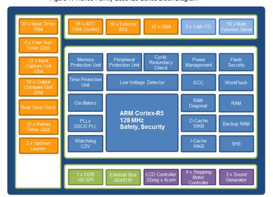
Figure 1. Traveo Family S6J3120 Series Block Diagram
