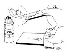
Preliminary dry abrading with 220- or 320-grit siliconcarbide paper is generally required if there is any surface scale or oxide. Final abrading is done by using 320-grit silicon-carbide paper on surfaces thoroughly wetted with M-Prep Conditioner A; this is followed by wiping dry with a gauze sponge. Repeat this wet abrading process with 400-grit silicon-carbide paper, then dry by slowly wiping through with a gauze sponge.
