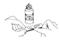
Now apply a liberal amount of M-Prep Neutralizer 5A and scrub with a cotton-tipped applicator. With a single, slow wiping motion of a gauze sponge, carefully dry this surface. Do not wipe back and forth because this may allow contaminants to be redeposited.
