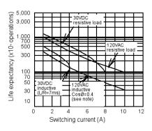
**Note:** Curve 120VAC inductive CosØ=0.4 is same for 250VAC resistive load.
