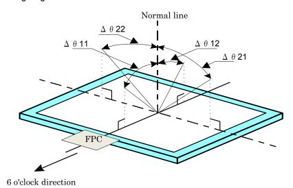
Figure 7-1 Defintion of Viewing Angle
