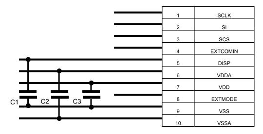
Figure 10-1 External capacitor recommendation capacity value
