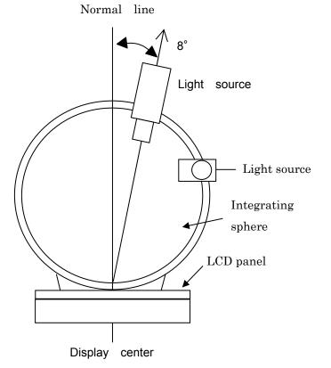
Figure 7-2 Contrast ratio, Reflection ratio, Panel chromaticity
