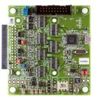
When connected to a DC9018A-B Evaluation/Development Mote, the DC9006 Eterna interface card provides a USB connection for both power and software access to the mote API UART port. The DC9006 comes with a DC9004 adapter card (not pictured) enabling the DC9006 to connect to the 10-pin programming and CLI header recommended for customer designs. Please see www.linear.com/solutions/3102 for more details.
