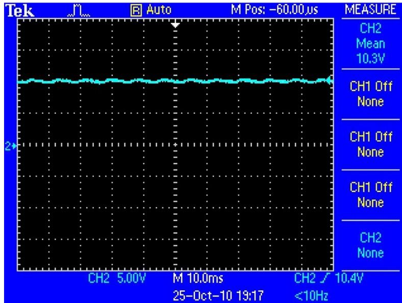
Connecting a 60 ohm resistor (~160 mA draw), it goes down to 10.3V
