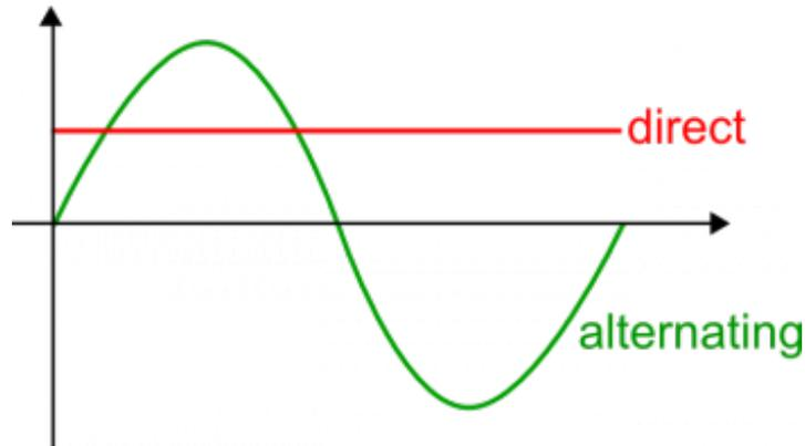
So the power coming out of your wall is high voltage AC but microcontrollers and servos and sensors all want low voltage DC. How shall we make it work? Converting between AC power and DC power requires different techniques depending on what the input and output is. We'll refer to this table:
