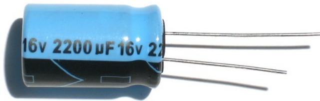
A capacitor **smooths** the voltage out, taking out the lumps, sort of how spring shocks in a car or mountain bike reduce the bumpiness of the road. Capacitors are great at this, but the big capacitors that are good at this (electrolytic) can't stand negative voltages - they'll explode!
