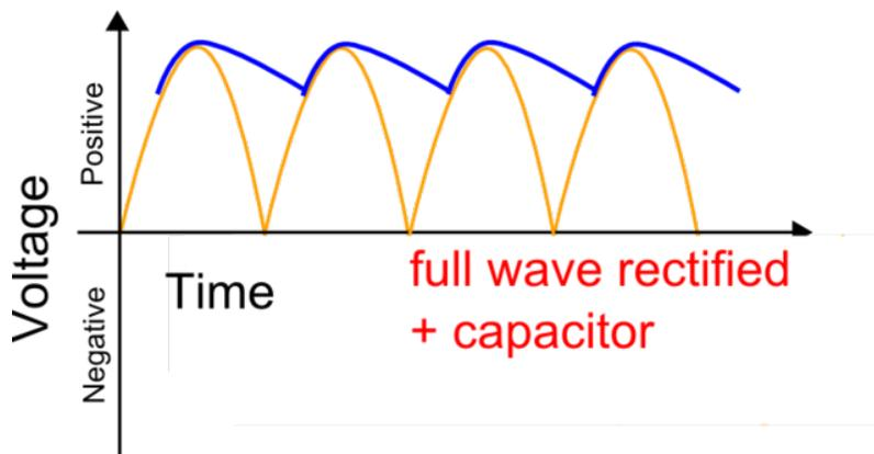
Basically, a full wave rectifier is way better than a half wave! So why even talk about half-wave type rectifiers? Well, because they're useful for a few other purposes. In general, you're unlikely to see an AC/DC converter that uses a half wave as the cost of the diodes makes up for the saving in capacitor size and cost!
