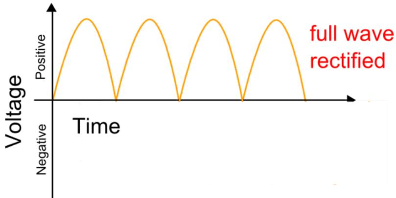
As you can see, there are twice as many humps - there isn't that "half the time, no voltage" thing going on. This means we can divide the calculated capacitor size to half of what it was in the previous.
