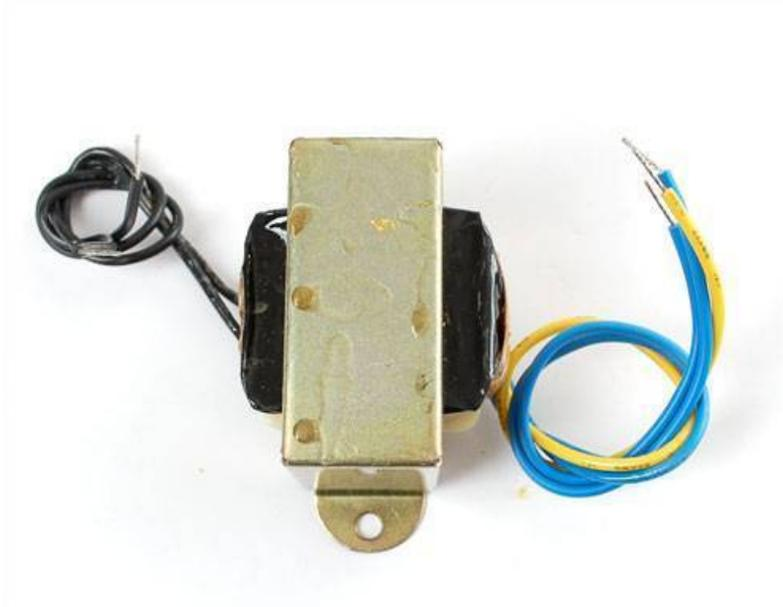
We aren't going to get into the heavy detail of the electromagnetic theory behind transformers except to say that they are made of two coils of wire around a chunk of iron. If the number of coils are the same on both sides then the AC voltage is the same on both sides. If one side has twice the coils, it has twice the voltage. They can be used 'backwards' or 'forwards'! For more detailed information, be sure to [check out the wikipedia page \(http://adafru.it/alf\)](http://adafru.it/alf).
