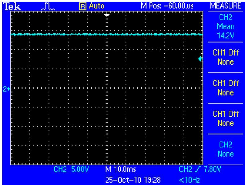
With no current being drawn on the supply, the voltage output is about 14V
