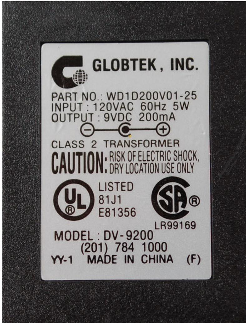
OK now that we've reviewed transformers, diodes when used as rectifiers and big capacitors, lets look at a chunky plugpack again. This time, we'll look inside by cutting it in half! This power supply is rated at **9VDC @ 200mA**.
