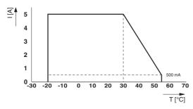
Figure 2 Vertical installation derating curve
