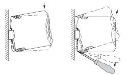
Figure 6 Mounting and removing
