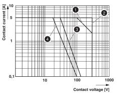
Figure 4 Relay load curve
