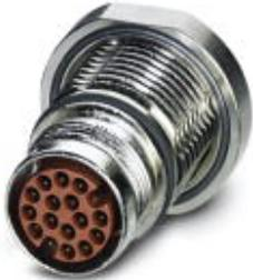
Device connector, rear mounting, straight, SPEEDCON locking, M17, Number of positions: 8, Type of contact: Male connector, Crimp connection, Axial O-ring, Central fixing, shielded: yes
