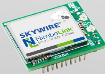
NimbeLink, a global leader in embedded cellular modem technology and asset tracking solutions, has created the Skywire NL-SW-LTE-QBG96 modem. This new Skywire modem offers LTE Category M/NB-IoT connectivity for global applications with fallback to 2G, as well as an integrated GPS/GNSS radio.
