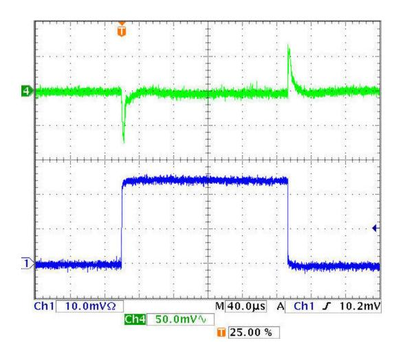
Figure 3. Load Step Response
