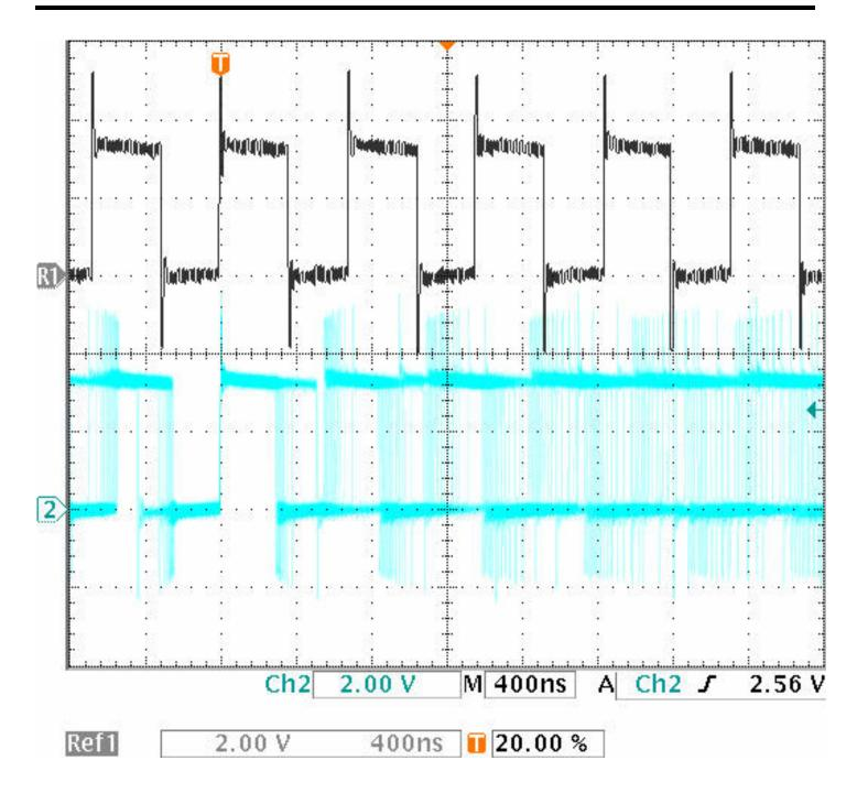
Figure 4. Normal Switching Operation vs. Spread Spectrum Operation  $V_{IN}-3.3V,\,V_{OUT}-1.8V,\,I_{OUT}-5A$
