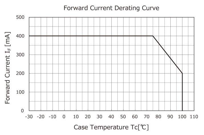
(Note) To keep the case temperature lower than the rating, enough heat-radiation performance needs to be secured by using an adequate heat sink (refer to section 7-③).
