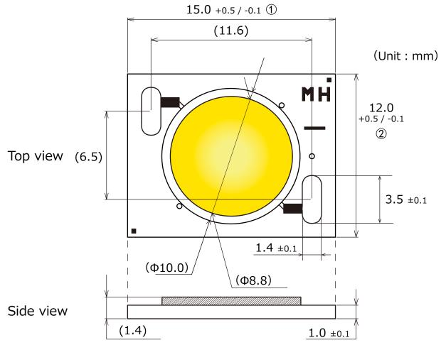
Values inside parentheses are reference values. External sizes of 1, 2 are determined by maximum dimensions, that include salient areas on the edges of respective sides.
