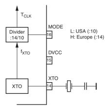
Pin MODE can now be set in accordance with the desired clock cycle  $T_{Clk}$ .  $T_{Clk}$  controls the following application-relevant parameters:
