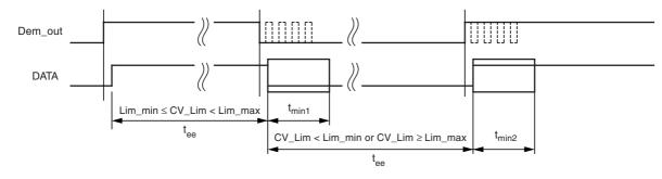
Figure 5-10. Steady L State Limited DATA Output Pattern after Transmission
