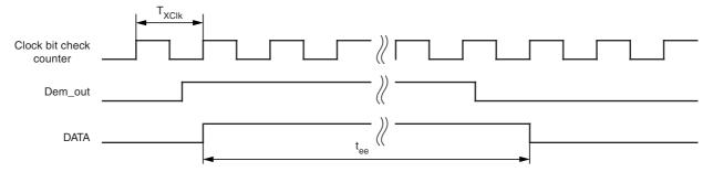
Figure 5-9. Debouncing of the Demodulator Output
