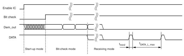
After the end of data transmission, the receiver remains active and random noise pulses appear at pin DATA. The edge-to-edge time period  $t_{ee}$  of the majority of these noise pulses is equal to or slightly higher than  $T_{DATA\_min}$ .
