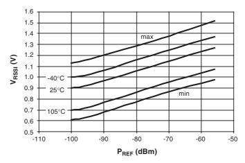
If  $R_{Sense}$  is connected to  $V_S$ , the receiver operates at a lower sensitivity. The reduced sensitivity is defined by the value of  $R_{Sense}$ , the maximum sensitivity by the signal-to-noise ratio of the LNA input. The reduced sensitivity is dependent on the signal strength at the output of the RSSI amplifier.
