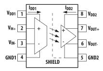
**NOTE** A 0.1  $\mu$ F bypass capacitor mus be connected between pins 1 and 4 and between pins 5 and 8.
