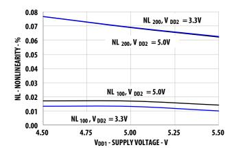
Figure 10 Nonlinearity vs. Supply V<sub>DD1</sub>
