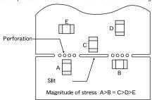
1-3. When breaking PC boards along their perforations, the amount of mechanical stress on the varistors can vary according to the method used. The following methods are listed in order from least stressful to most stressful: push-back, slit, V-grooving, and perforation. Thus, any ideal SMD varistor layout must also consider the PCB splitting procedure.
