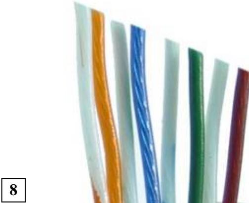
Trim off the wire ends at an angle to facilitate loading the wires into the load bar.
