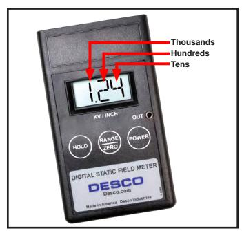
Figure 6. Reading the Digital Static Field Meter while in the ±20 kV range
