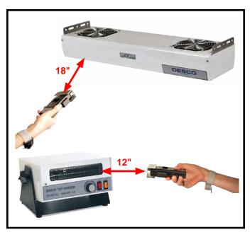
Figure 5. Auditing ionization equipment with the Digital Static Field Meter and Conductive Plate (Ref: ANSI/ESD SP3.3)
