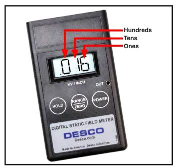
Figure 7. Reading the Digital Static Field Meter while in the ±2 kV range
