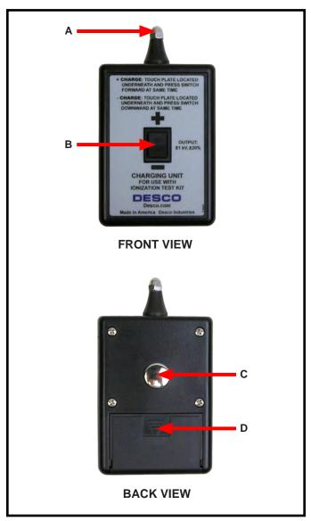
Figure 3. Charger features and components
