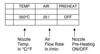
In the Manual operating mode the parameters for the nozzle temperature, air flow rate and switching on or off the pre-heating can be set.
