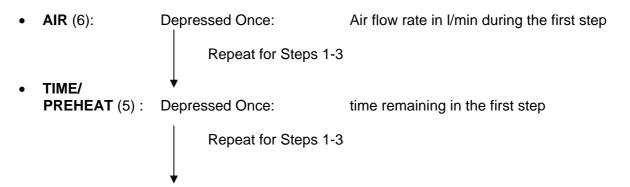
The active value is marked on the display and can be changed using the  ${\bf UP}$  /  ${\bf DOWN}$  (2) / (3) Control Keys. Keeping the Control Key depressed, rapidly changes the value.
