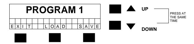
The program memories 1 - 10 can be selected using the **UP/DOWN** Control Keys (2)/(3).
