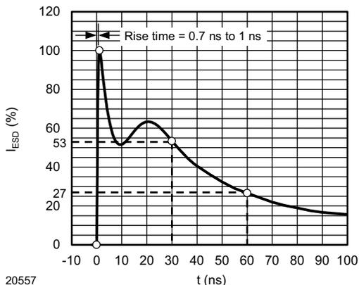
Fig. 1 - ESD Discharge Current Wave Form
