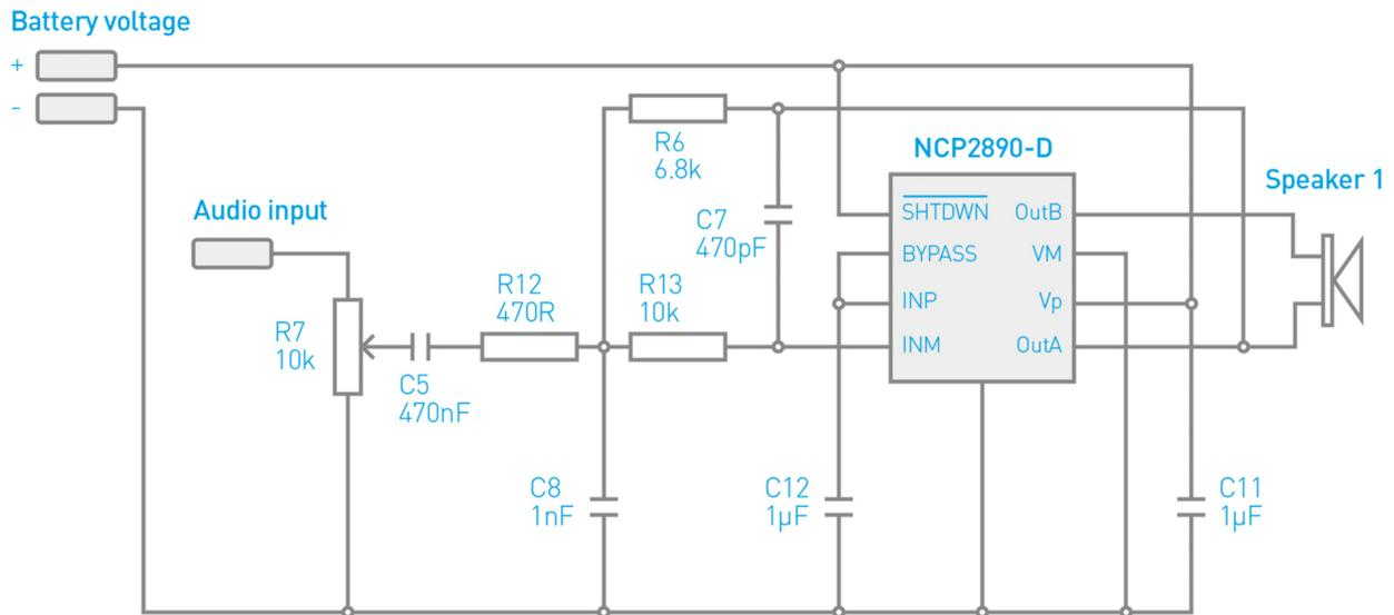
The audio amplification is performed by another Integrated Circuit or IC called an NCP2890-D. Inside the NCP2890-D are lots of transistors, which are connected together to allow the small input signal to be amplified into a more powerful output that can drive a speaker.
