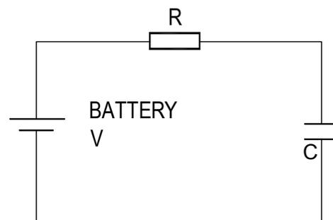
When a capacitor is connected to an item such as a battery, charge will flow from the battery into it. Therefore the capacitor will begin to fill up. The flow of water in the picture above left is the equivalent of how the electrical charge will flow in the circuit shown on the right.
